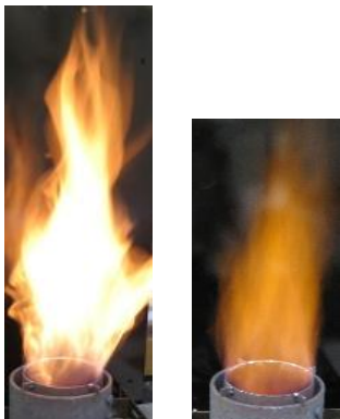
Fuel 100% Water 50vol% Fig.2 Burner flame
